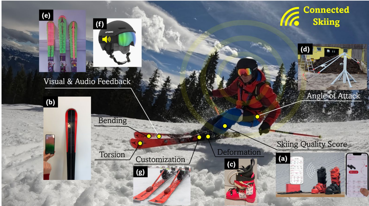
Figure 1: Overview of developed prototypes and demonstrators: (a) Connected Boot with companion app; (b) PyzoFlex® ski instrumented for bending and torsion sensing; (c) PyzoFlex® Boot for measuring ski boot deformation; (d) GNSS-based prototype on a ski simulation rig; (e) SkiTip display; (f) real-time sonification toolkit (SkiTone); (g) magnetorheological ski (MR-Ski) that enables real-time adjustment of the ski's mechanical properties (Author's own figure).
